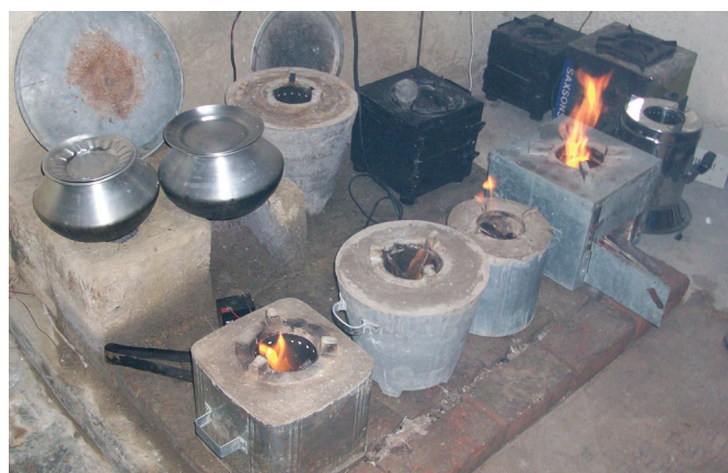
Several types of advanced cookstoves are tested as part of a project by The Energy and Resources Institute (TERI) in Jagdishpur, northern India.
