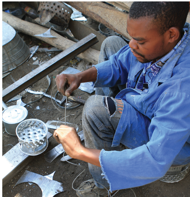
A local finsmith in Zambia makes small cookstoves by hand. Low-cost local production can help improved cookstove projects’ chances of success.
