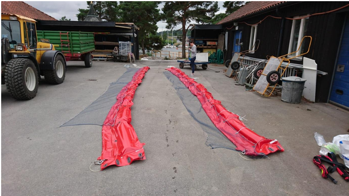
Figure 1. Litter booms (C500) equipped with net curtains.
