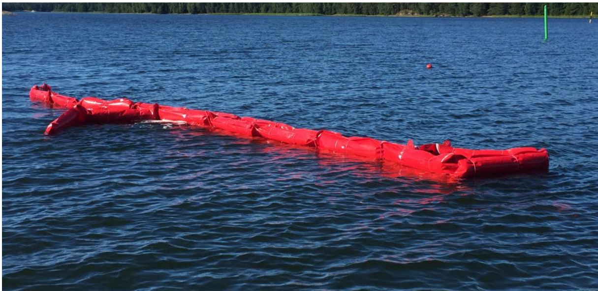
Figure 16. One mooring point of Boom 1 came out of position resulting in a deformation of the litter boom. It was not able to capture any litter.
