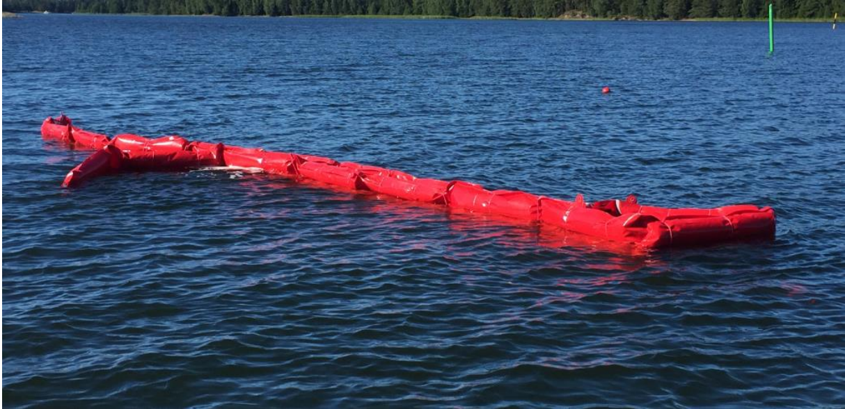
Figure 3. Strong winds resulted in a deformation of the litter boom. It was not able to capture any litter.
