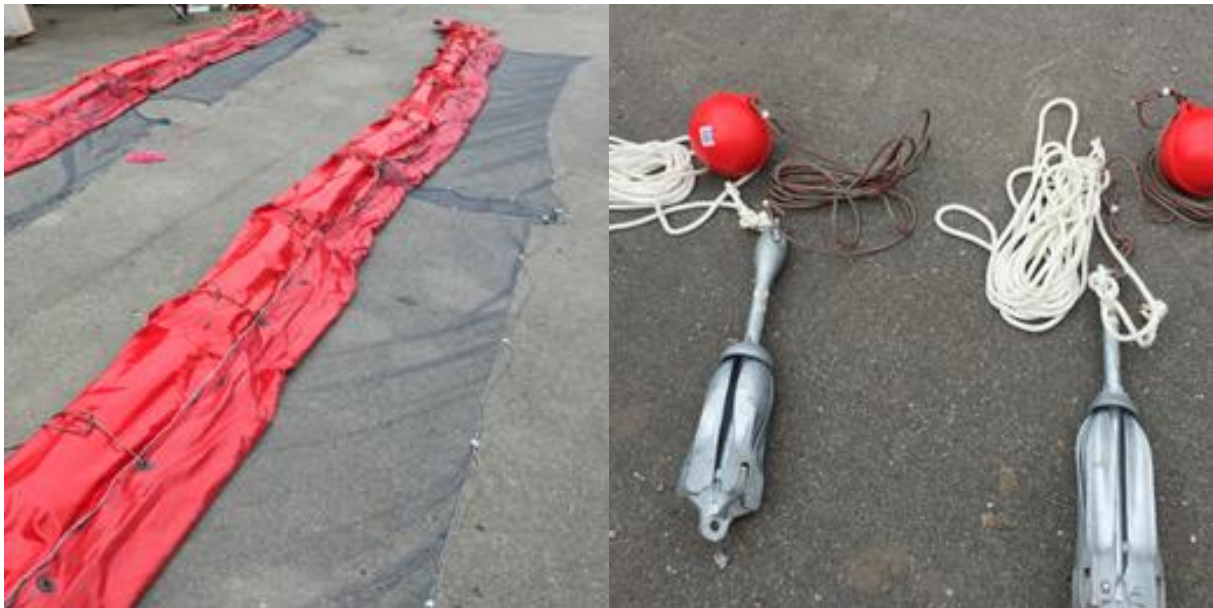
Figure 2. Litter booms with net curtains and grapnel anchors used to moor the litter boom.
