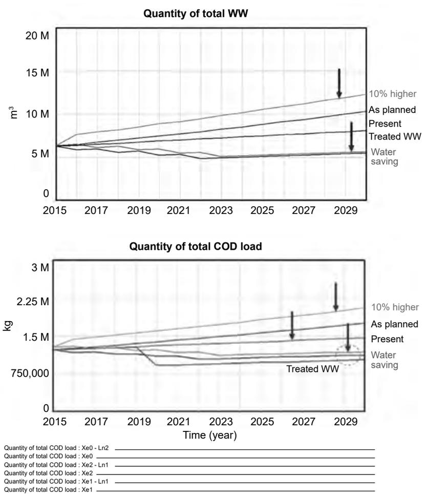
Figure 13.13. Changes in wastewater quantity and COD load under the six scenarios in the study area’s water drainage network in 2030
