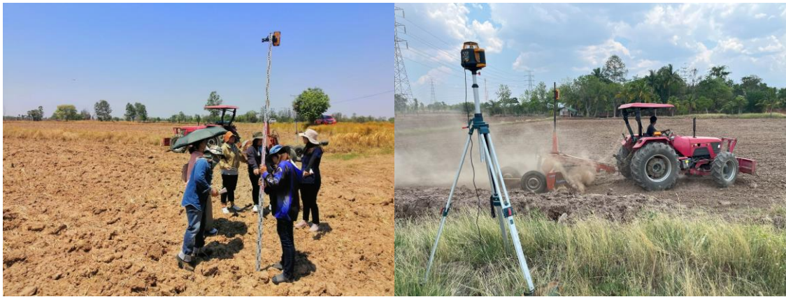
Photo 3: Site at Phimai District, Nakhon Ratchasima (a) Farmer using laser guide to measure in the field, and (b) laser land leveling
